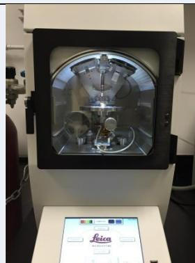
**Figure 4:** Sputter system for carbon and iridium coating for SEM sample prep.
