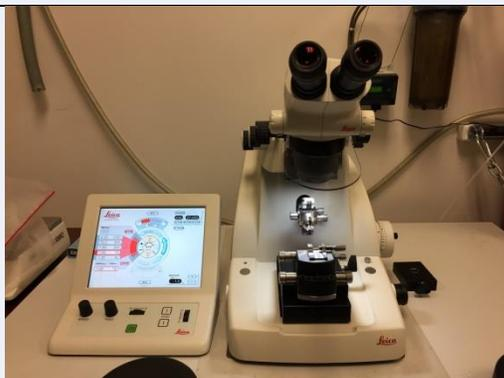
**Figure 3:** Microtome with cryo-capability for TEM sample prep.
