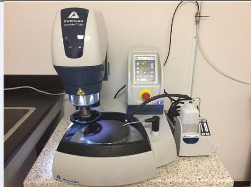
**Figure 2:** Grinding and polishing machine for microscopy sample prep.
